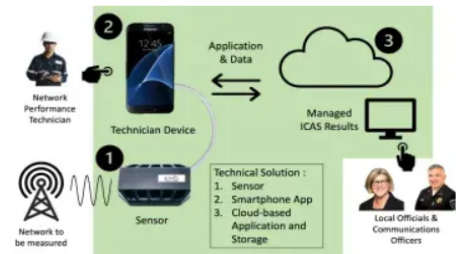
A diagram of the PRISM In-building Coverage Analysis System Process. Photo credit: Epiq Solutions.
