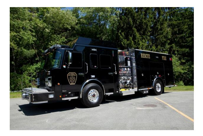
This vehicle is the primary attack apparatus for fire suppression, auto accidents, and hazardous material emergencies. It comes with a 2000 GPM pump, 750-gallon tank, foam capabilities, deck gun, multiple pre-connected, extrication equipment, and a light tower.
