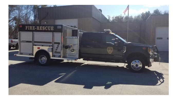
This vehicle is used for fire suppression, auto accidents, hazardous material emergencies; and is backup apparatus for medical/trauma emergencies. It comes with a 1500 GPM pump, 300-gallon water tank, multiple pre-connected hose lines for rapid deployment.
