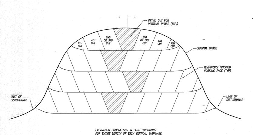
DETAIL SHOWING "DOWNCUTTING" EXCAVATION METHOD
