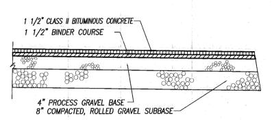
BITUMINOUS CONCRETE PAVEMENT NOT TO SCALE
