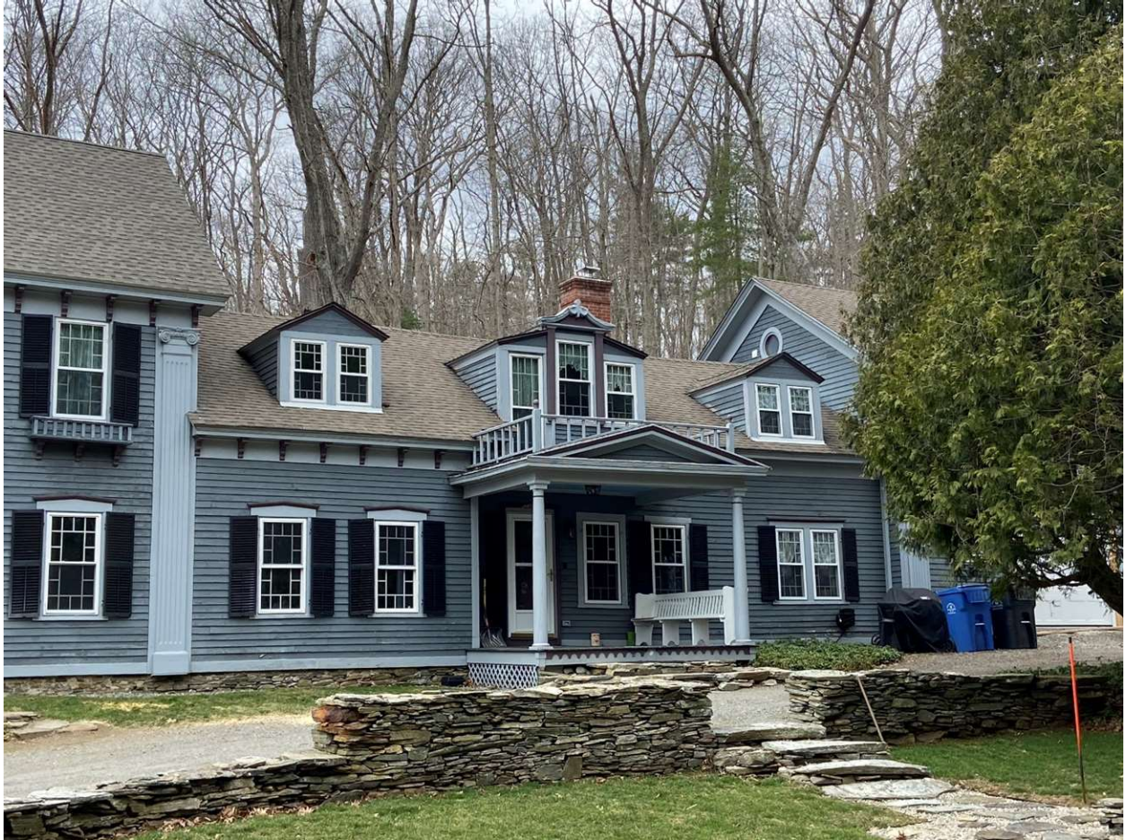
Current view of middle of house – proposed new full dormer and new foyer roof (see drawing) New mini split condensers to be placed in front of column between sections on the left and between window sets to right of porch. Both to be screened with lattice and climbing rose bushes.
