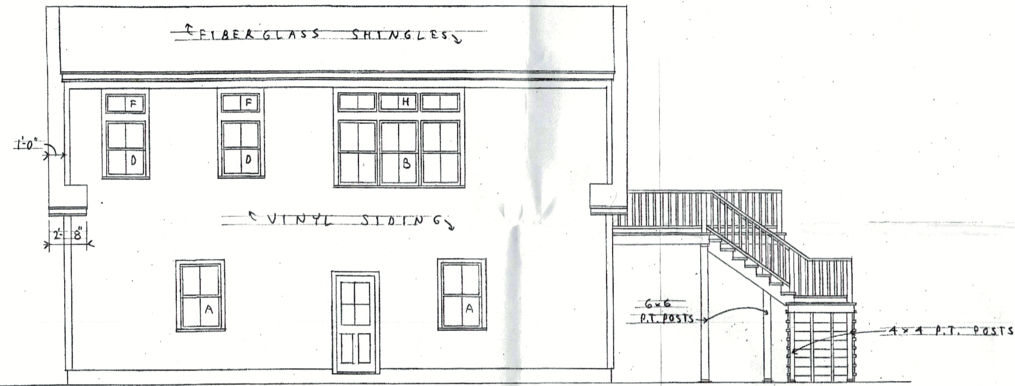
REAR ELEVATION SCALE: 1/4" = 1'-0"
