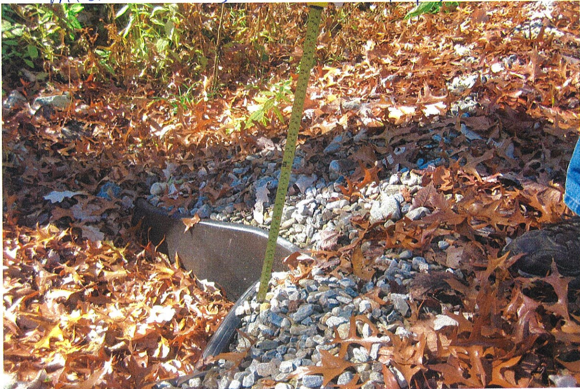
Tape measured 9" of fill over third pipe in middle crossing (westernmost pipe)
