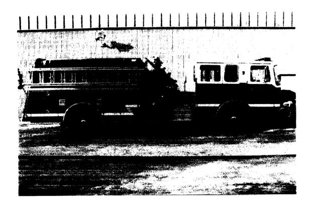
This vehicle is used for fire suppression, auto accidents, hazardous material emergencies, and is backup apparatus for medical/trauma emergencies. It comes with a 1500 GPM pump, 1000 gallon tank, foam capabilities, multiple pre-connected hose lines for rapid deployment of large amounts of water.
