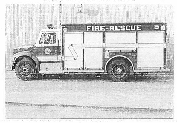
This vehicle is used as first due to medical/trauma emergencies, operates as rehab unit and cascade operations at fire scenes, currently carries secondary extrication equipment, and fire support equipment as well as hazardous materials equipment.
